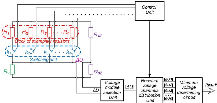
Fig. 1. Schematic model of subsystem
