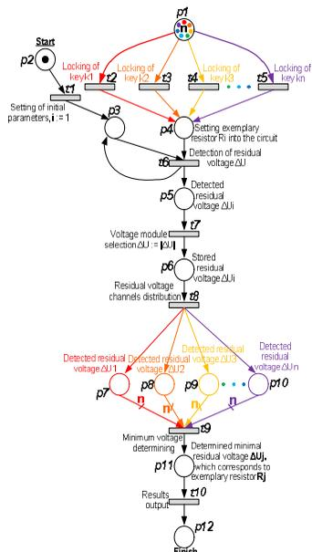
Fig. 3. Functional model, based on colored Petri nets
